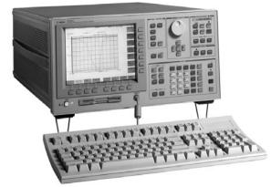
The 4156C Precision Semiconductor Parameter Analyzer provides highly accurate laboratory bench top parameter analyzers for advanced device characterization. The superior low-current and low-voltage resolution and built-in quasi-static CV measurement capability of the 4156C provide a firm foundation for future expansion with other measurement instruments. The 41501B Expander can extend your capabilities to 1 A/200 V as well as supporting dual pulse generator units (PGUs) and a 1.6 A ground unit.
